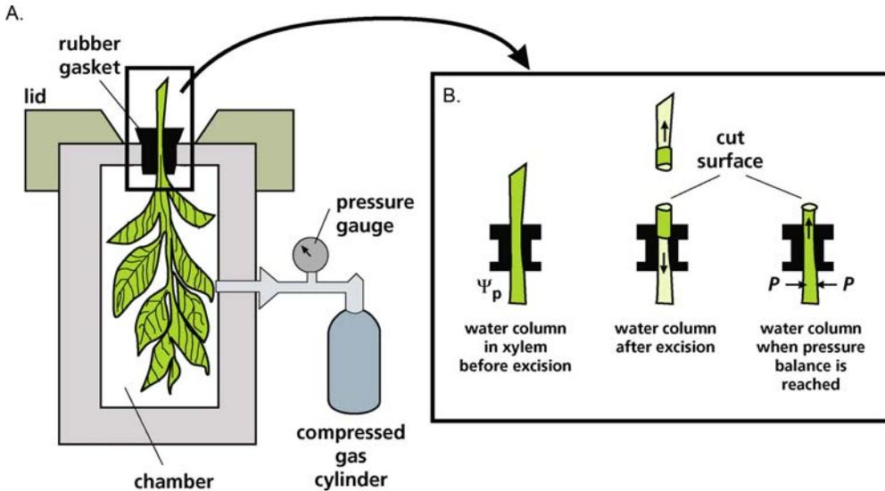
FIGURE 13. (Left) Schematic representation of the Scholander pressure chamber that is used for the measurement of negative hydrostatic pressures in the xylem ( $\Psi_p$ ). A cut shoot, twig, root, or leaf is excised, and the negative  $\Psi_p$  in the xylem causes the water column to be drawn into, e.g., the leaf. (Right) A leaf (or other plant part) is mounted in a gasket and placed in the pressure chamber with the cut end protruding through the lid.
