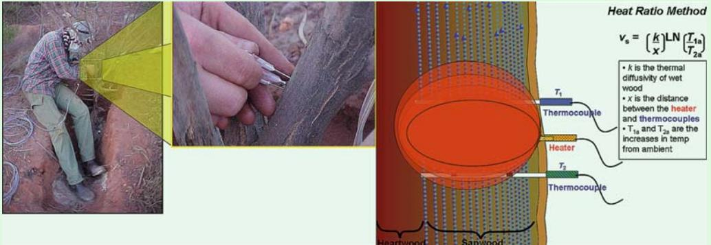
**FIGURE 1.** Sap-flow measurements using the heat-ratio method require insertion of probes in a stem, root, or branch (*left*). The middle probe is a heater, the other ones are thermocouples. If sap moves upward, then the heat pulse will reach the upper
